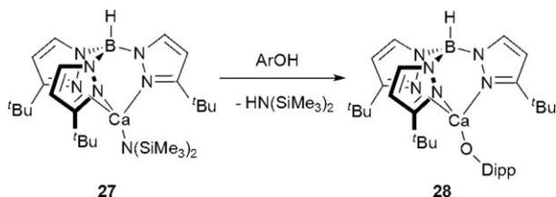
**Scheme 4** Synthesis of a calcium aryloxy complex of the TPB ligand.
