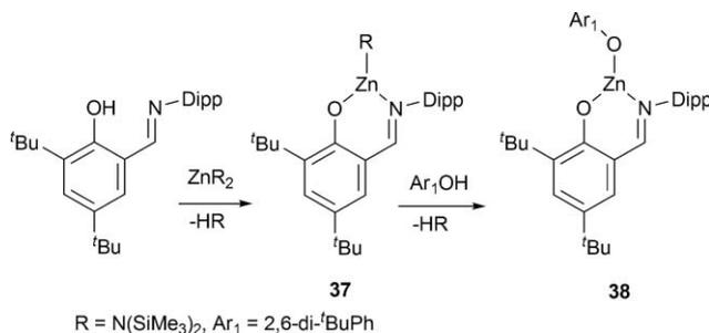
**Scheme 8** Synthesis of zinc amide (**37**) and aryloxide (**38**) complexes of a Schiff base ligand.
