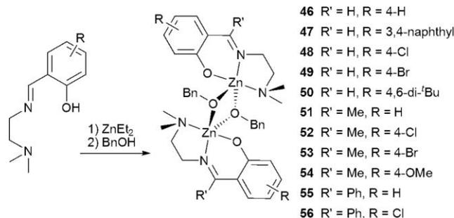
**Scheme 11** Preparation of zinc alkoxide complexes of a tridentate Schiff base ligand.
