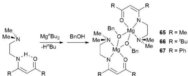
**Scheme 12** Synthesis of magnesium alkoxide complexes supported by a ketiminate ancillary ligand.
