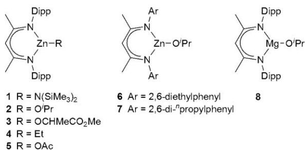
**Fig. 2** General structure of single-site catalysts prepared from the BDI ligand framework.
