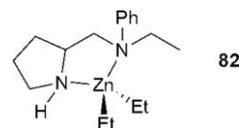
**Fig. 13** Proposed structure of a diethylzinc complex (**82**) of the neutral pyrrolidine ligand.
