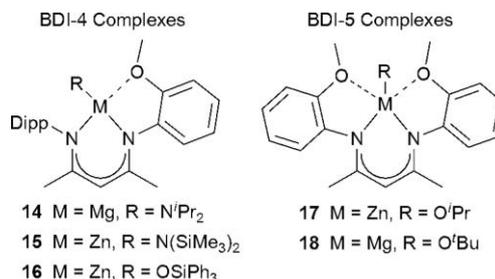
**Fig. 4** Magnesium and zinc complexes prepared from modified BDI ligands bearing ether substituents.
