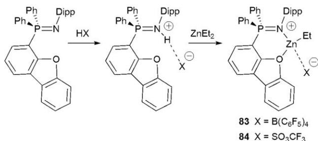
**Scheme 18** Synthesis of activated zinc ethyl complexes by protonation of the DBF ligand followed by reaction with diethylzinc.
