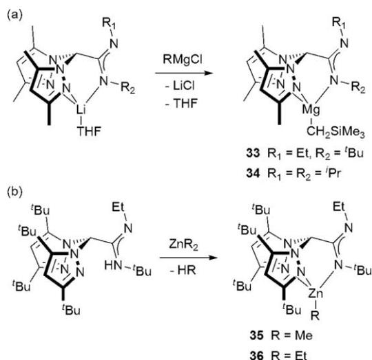
**Scheme 7** Preparation of (a) magnesium and (b) zinc complexes of HSC scaffolds.
