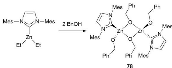
**Scheme 16** Preparation of an NHC supported zinc alkoxydimer (**78**).
