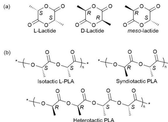
**Fig. 1** (a) Lactide monomer stereoisomers. (b) Microstructures of poly(lactide) which can be achieved either through polymerization of optically pure L-lactide (L-PLA) or by stereochemically selective polymerization of *rac*-lactide or *meso*-lactide (heterotactic and syndiotactic PLA, respectively).
