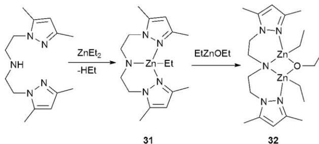
**Scheme 6** Synthesis of the BPA supported mononuclear zinc ethyl complex **31** and the binuclear zinc alkoxide **32**.
