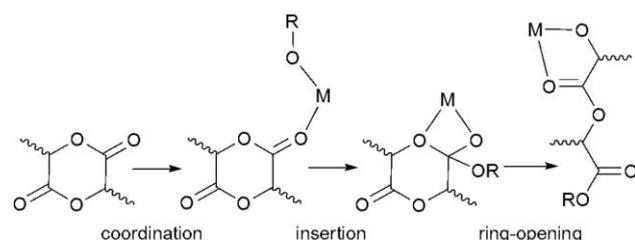
Scheme 2 General coordination–insertion mechanism for the metal-catalysed ring-opening polymerization of lactide.
